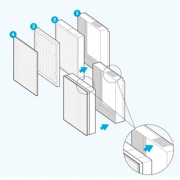
» Remove all filters from plastic. Check that the Velcro on the carbon filter is facing out. Attach pre-filter to the Velcro strips in each corner of the carbon filter.
