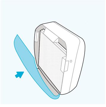
» Place filter assembly back into unit. White sticker on top and white pre-filter in front.
