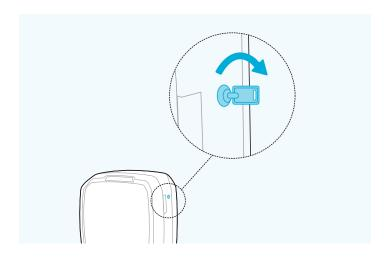
» Once settings are complete, insert key on the right side and rotate clockwise ¼ turn to lock machine.
