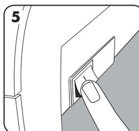
5 Switch the machine on using the power switch located at the rear of the machine.
