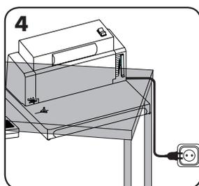
4 Plug the machine into an easily accessible mains socket. Switch the mains supply on.
