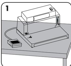
1 Ensure the machine is on a stable surface.
