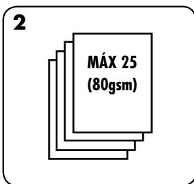
Punch sheets in small batches so as not to overload the machine or the user.
