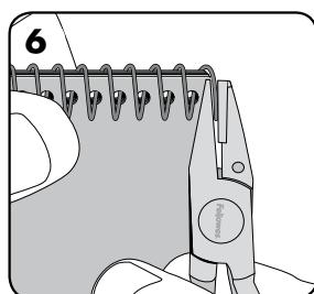
Use the binding pliers to cut and fold the end of the metal coil. Clip off the excess coil.
