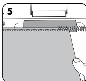
Hold the document in both hands, with the metal coil on the right side. Touch the metal coil against the inserting roller to bind the document.
